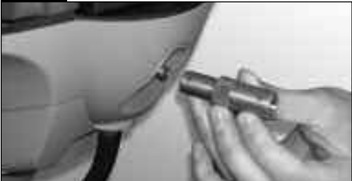
First hand-screw the Quick Clear adapter onto the valve.
